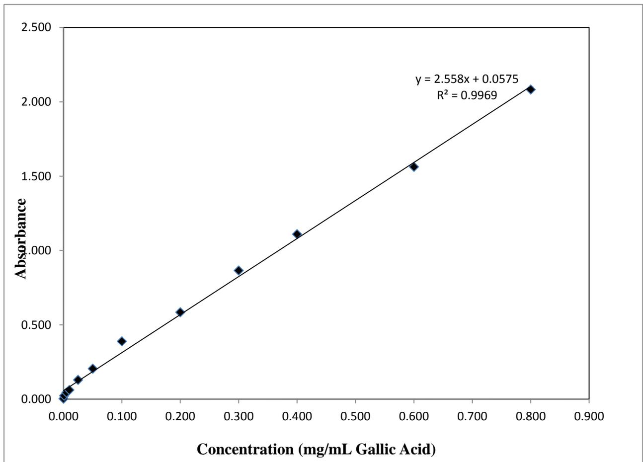
**Figure 8.0 Standard Calibration Curve of Gallic Acid for TPC Quantitation**
