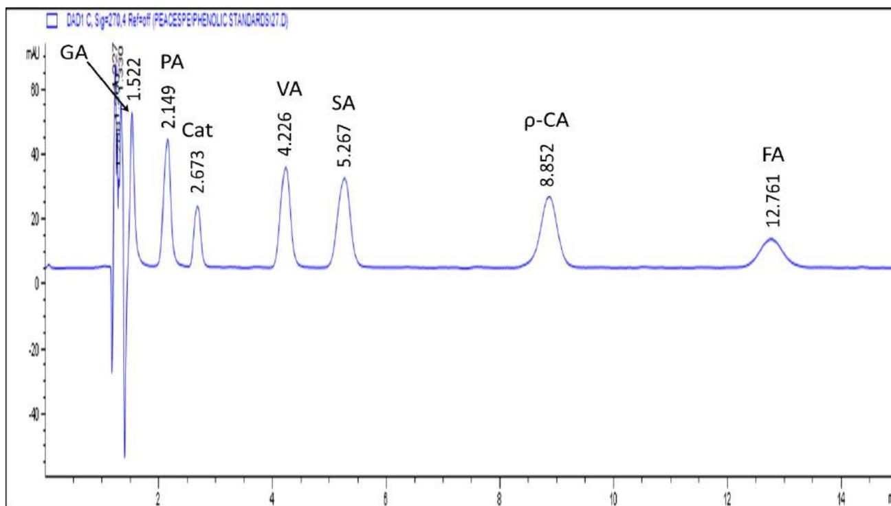
**Figure 5.0 Representative Chromatogram of the Phenolic Standard Mixture detection at 270nm**
