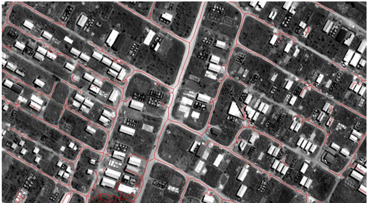
Figure 13 Overlay of line vector format of unpaved roads and the original subset image of a panchromatic image.
