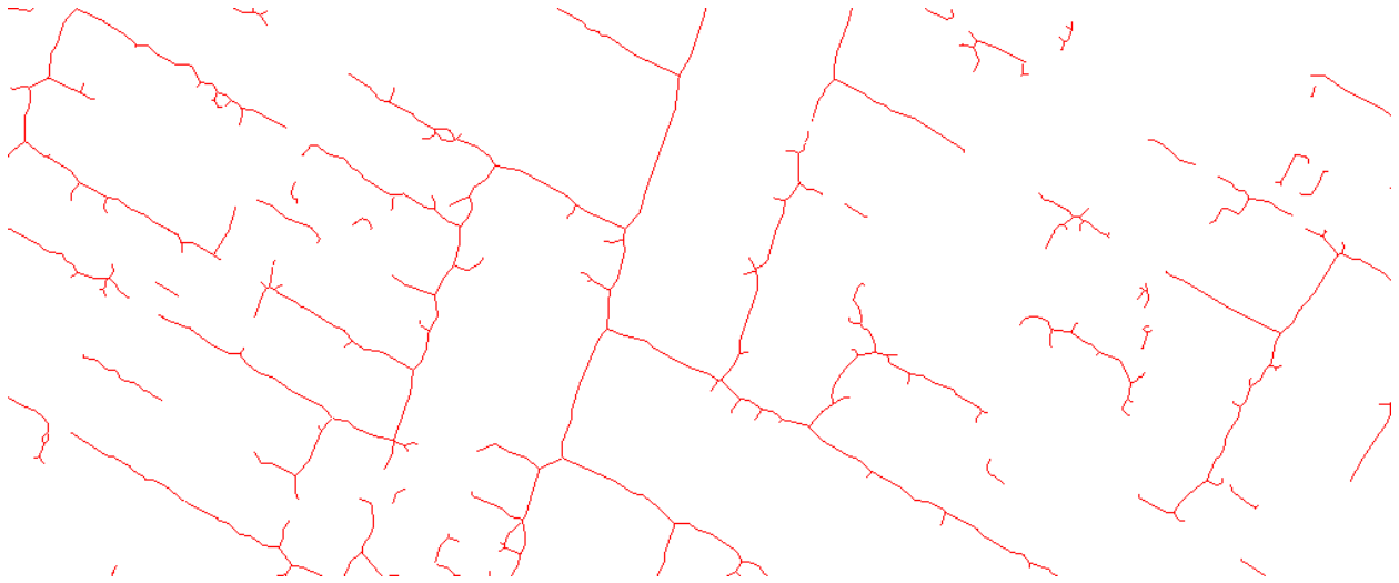
Figure 12 Vector line format of extracted unpaved roads from a panchromatic image.
