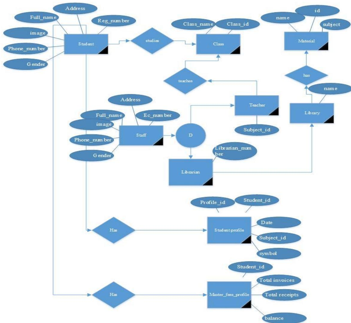
**Figure 4.5 Enhanced entity relationship diagram**
