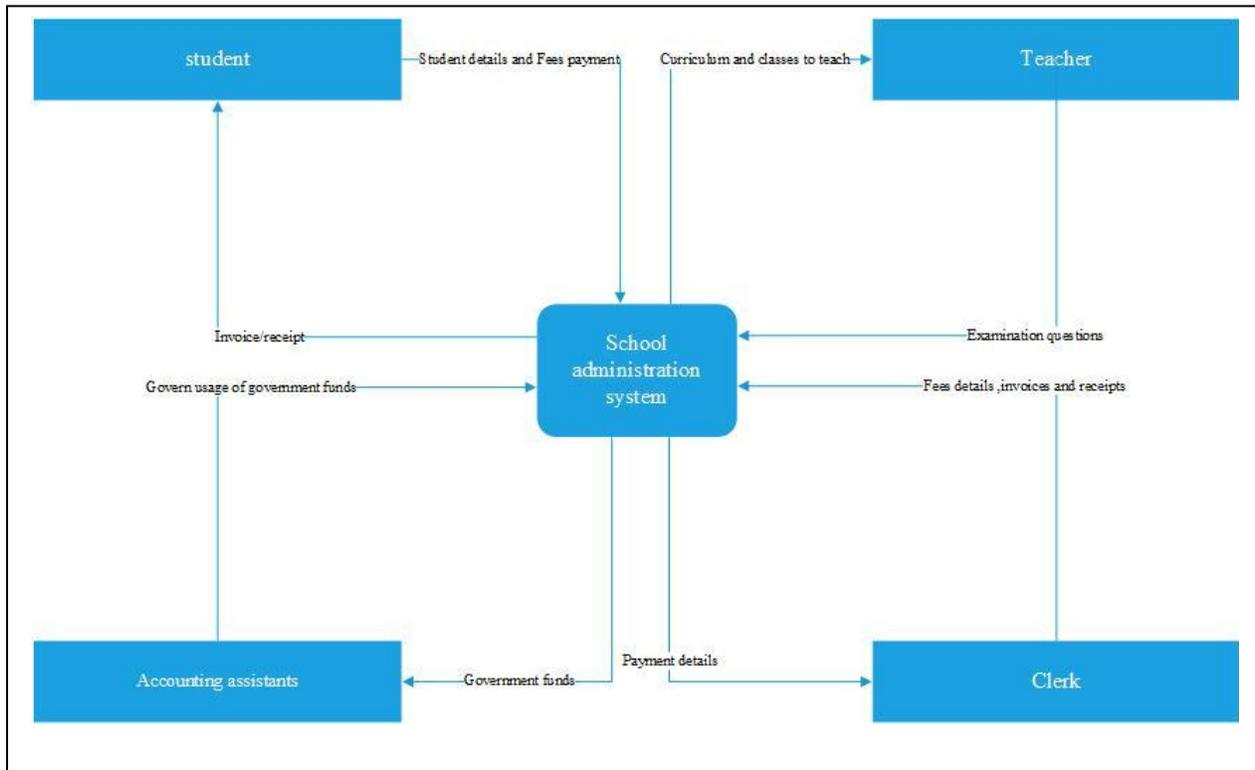
**Figure 3.2 Context Diagram of current system**
