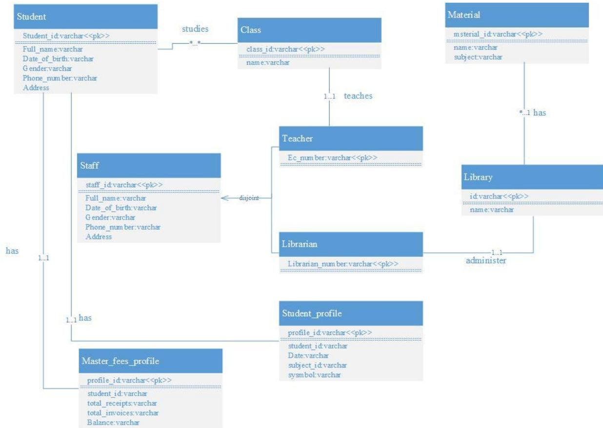
**Figure 4.7 Class diagram**
