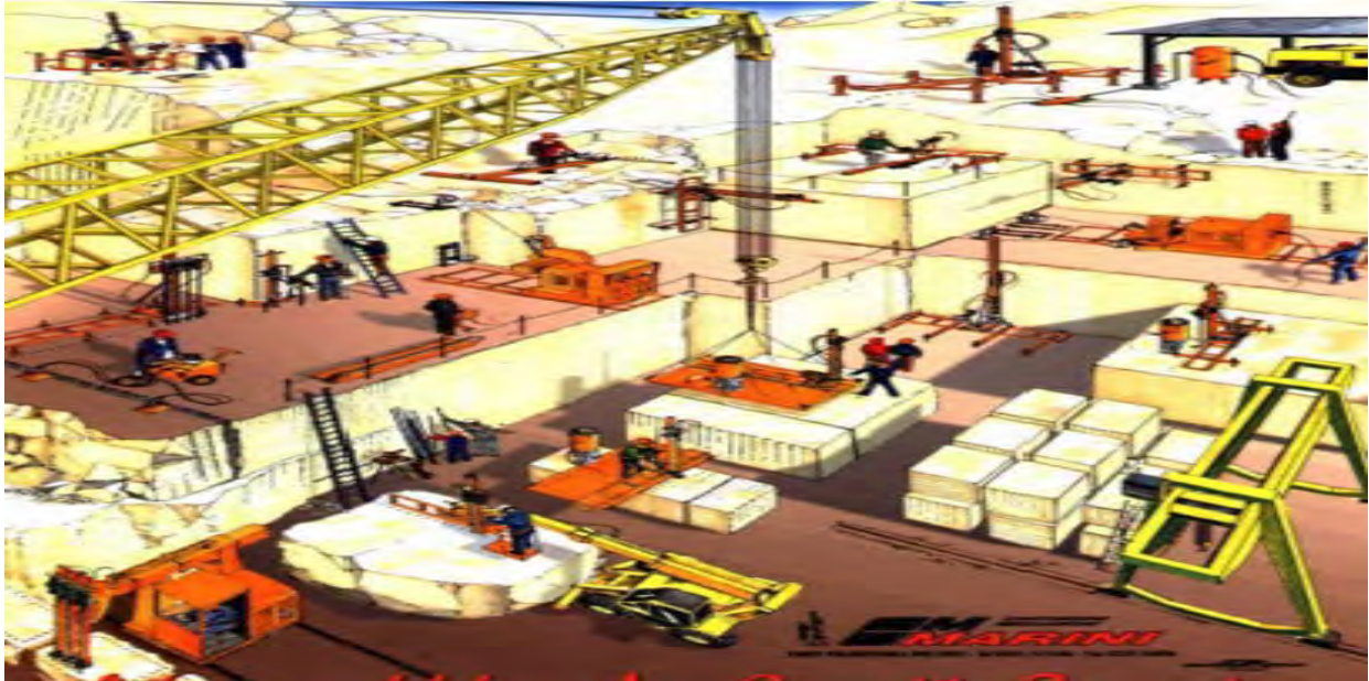
Plate 2.1 a granite quarry operation, using wire saws, drills, and other support equipment for extraction. Source: Bourque and Associates (1991).
