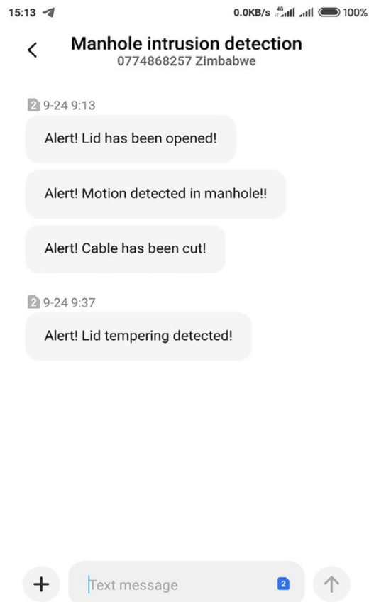
Fig. 6. Snapshot of mobile phone notification messages sent by the proposed system.
