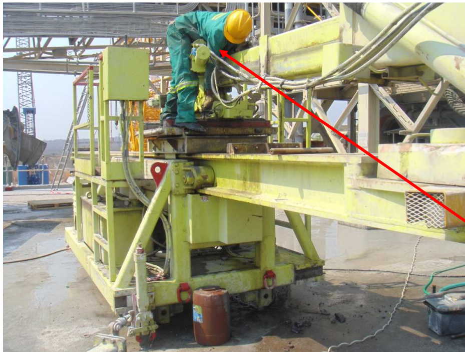
Plate 4.5: Contractor repairing a liner machine. Source: Primary data.
